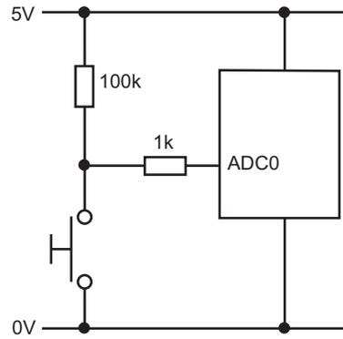
Note that the 1k is essential to prevent a possible short circuit situation (if the switch was pushed whilst the hibernate starts, as it will momentarily make ADC0 an output to 'charge the capacitor').
