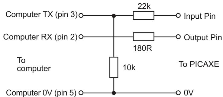
**PICAXE-08/08M/14M** - Due to the internal structure of input3 on these chips, a 1N4148 diode is required between the pin and V+ for serin to work on this particular pin ('bar' end of diode to V+) with this circuit. All other pins have an internal diode.
