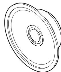
For richer sounds a speaker should be used. Once again the quality of the sound-box the speaker is placed in is the most significant factor for quality of sound. Speakers can be driven directly (using a series capacitor) or via a simply push-pull transistor amplifier.
