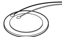
The best piezo sound comes from the 'plastic cased' variants. Uncased piezos are also often used in schools due to their low cost, but the 'copper' side will need fixing to a suitable sound-board (piece of card, polystyrene cup or even the PCB itself) with double sided tape to amplify the sound.
