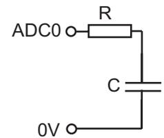
**MANUAL WAKEUP** - The capacitor can also be completely replaced by a push-to-make switch (use 1k resistor as R and add another 100k resistor from the top of the switch to V+ to act as a positive voltage pull-up). The switch then acts as a manual 'wake-up' switch.
